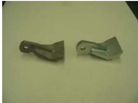
Figure 6: Machined and Cast Operational Evaluation Cutters
