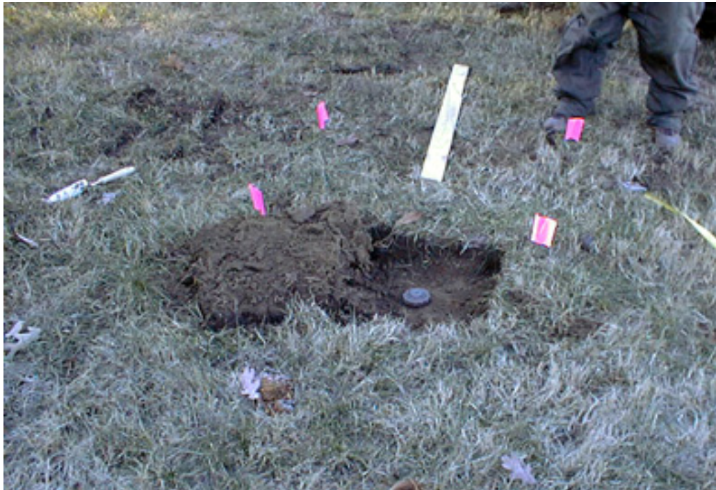
4.2.1 Effect of Vegetation Cover FIGURE 5. MKII Mine Burial in Sod
