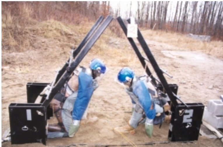
Figure 1. Test set-up showing mannequins in kneeling-on-one knee position wearing Sport helmets and a Demining Ensemble, held in position by test apparatus. Mannequin 1 (on left) is positioned with nose 0.80 m from mine, while mannequin 2 is positioned with nose 0.70 m from mine.
