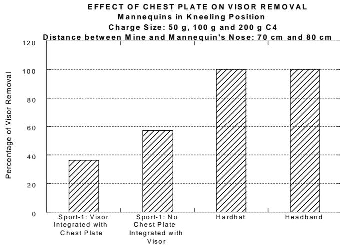
Figure 6. Percentage of visors removed from face during blast, illustrating effect of overlapping chest plate and properly mounted visor.
