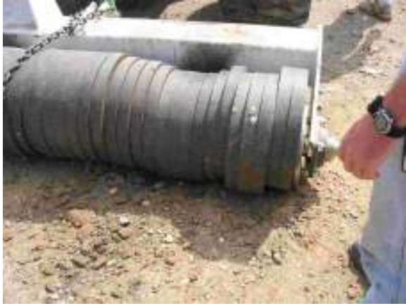
Figure 23: Results of Blast Test Against Roller
