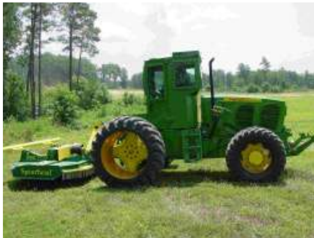
Figure 1: Mine Clearing/Survivable Vehicle (MCSV) with Rotary Mower
