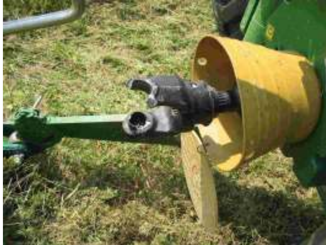
Figure 21: Sheared Universal Joint
