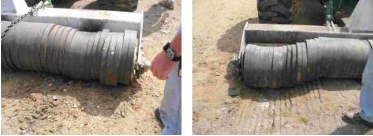
Figure 23: Results of Blast Test Against Roller
