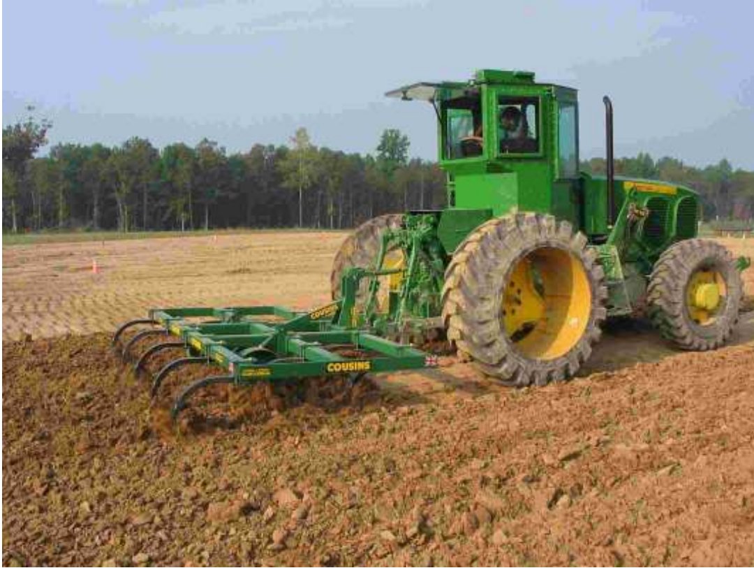
Figure 26: Spring Tine Cultivator Demonstration
