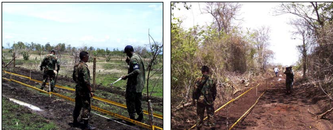
Figure 3. Construction of the 1-m by 20-m test lanes, the black soil lane (left) and the red soil lane (right). (NOTE: The black soil lane can be seen further down the road in the red soil lane picture (right), showing the near proximity of the lanes.)
