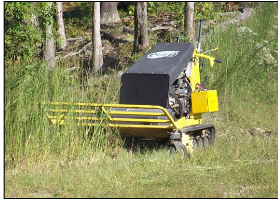
Figure 1: Peco Tracked Brush Blazer TBB-2001
